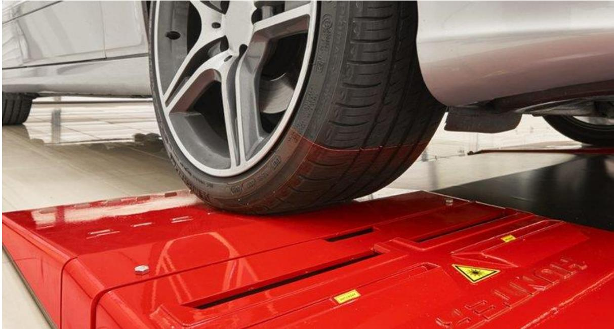
*The Hunter Engineering Quick Tread™ ramp incorporating the TreadReader™ tyre measurement sensor*
