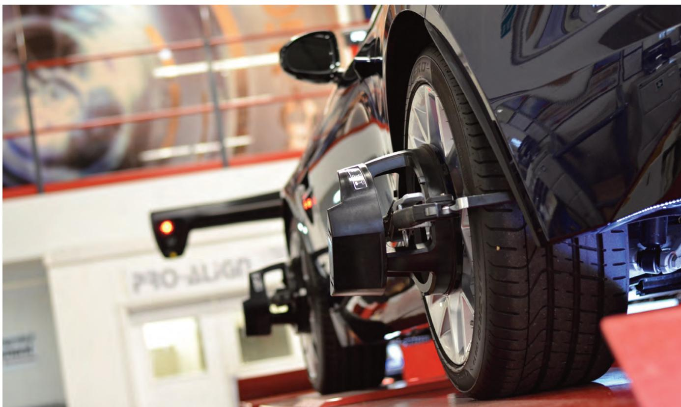
**V**ehicles are becoming increasingly safe thanks to technology, but for garages the price is the need to work to an even more precise standard. Accurate wheel and body alignment is now an absolute necessity so that a host of systems function correctly. Properly marketed, wheel and body alignment can also be a great profit centre too.
